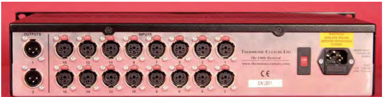
The rear panel of the Little Bustard. Despite the presence of XLRs, the inputs are unbalanced — because designer Vic Keary believes this configuration sounds better.
